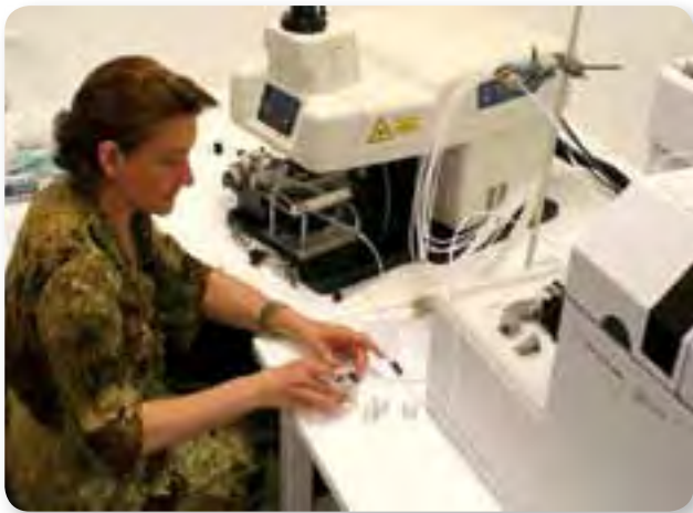
Laboratory Analyst, Elena Lounejeva, operating the New Wave UP213 laserprobe.
