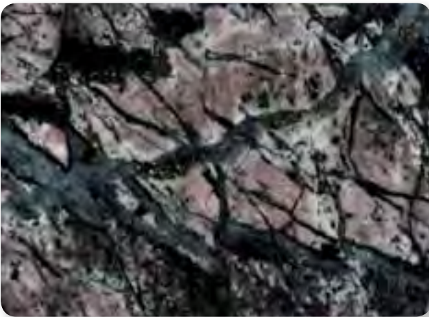
Rock from Golpu porphyry deposit containing quartz-orthoclase-biotite-magnetite-calcopyrite.
