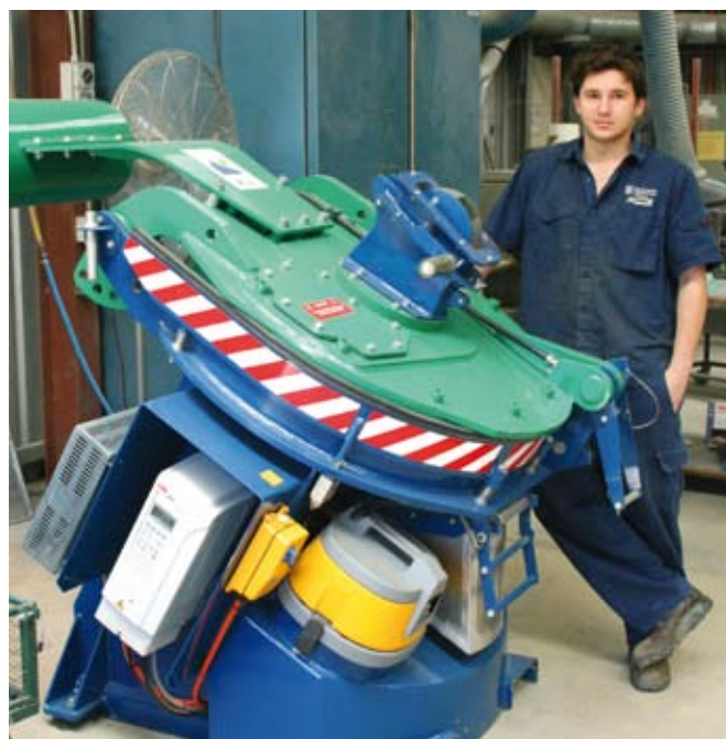
Pat Walters with an RBT device for rapid hardness testing at the Julius Kruttschnitt Mineral Research Centre at the University of Queensland.
