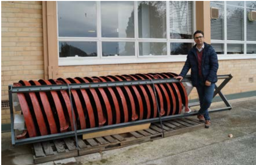
Dr Mohammad Fathi with one of the pieces of lab equipment that was acquired in 2024. This spiral will be used for gravity separation-based preconcentration processes for scheelite.
