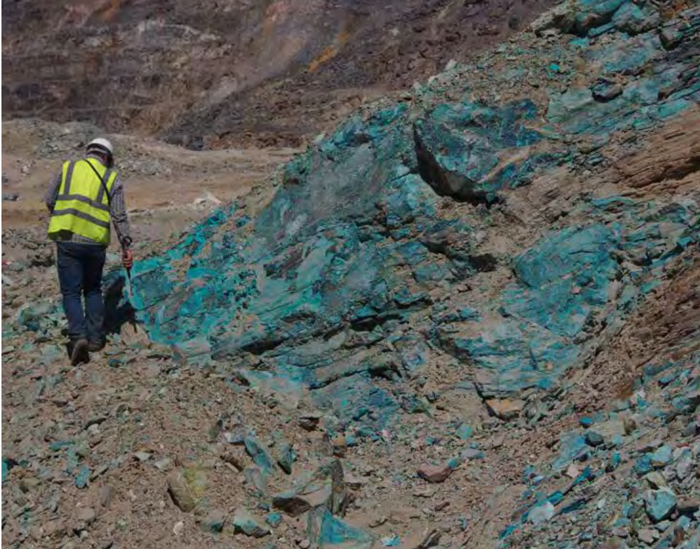
PhD student Jacob Heathcote inspects supergene ore in Kansanshi main pit, NW Zambia. Jacob is investigating the relationship between gold and copper in primary and supergene ores at the mine.
