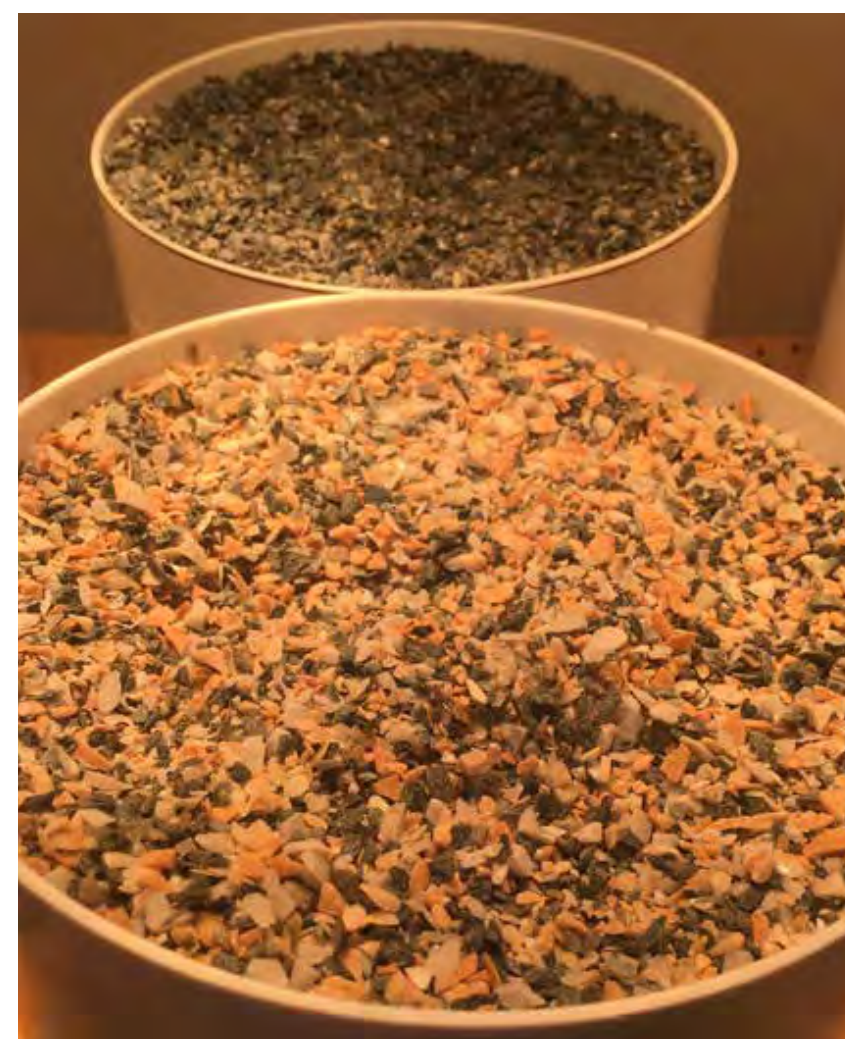
FROM TOP: Geoenvironmental characterisation of waste rock using the net acid generation test; Kinetic cell.
