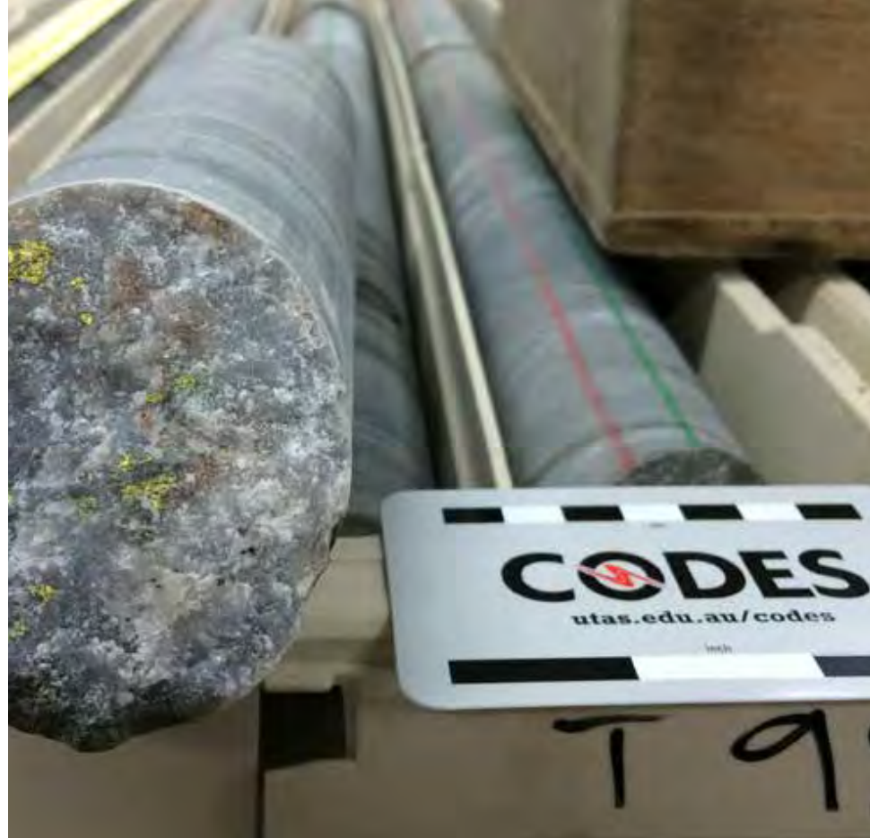
FROM LEFT: High resolution hyperspectral images of drill core are collected using Corescan's automated system; Chalcopyrite on a broken quartz vein surface.
