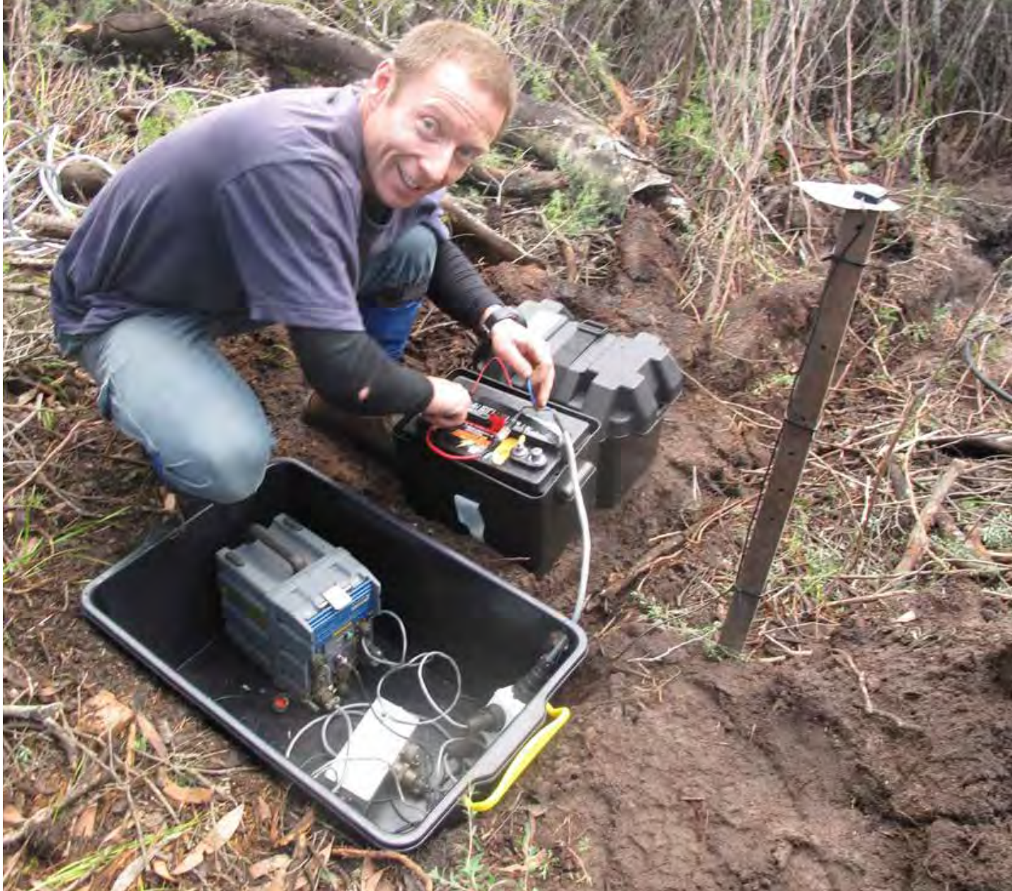
Collaborator, Andy Wakefield, from Mineral Resources Tasmania, installing passive seismic array equipment.
