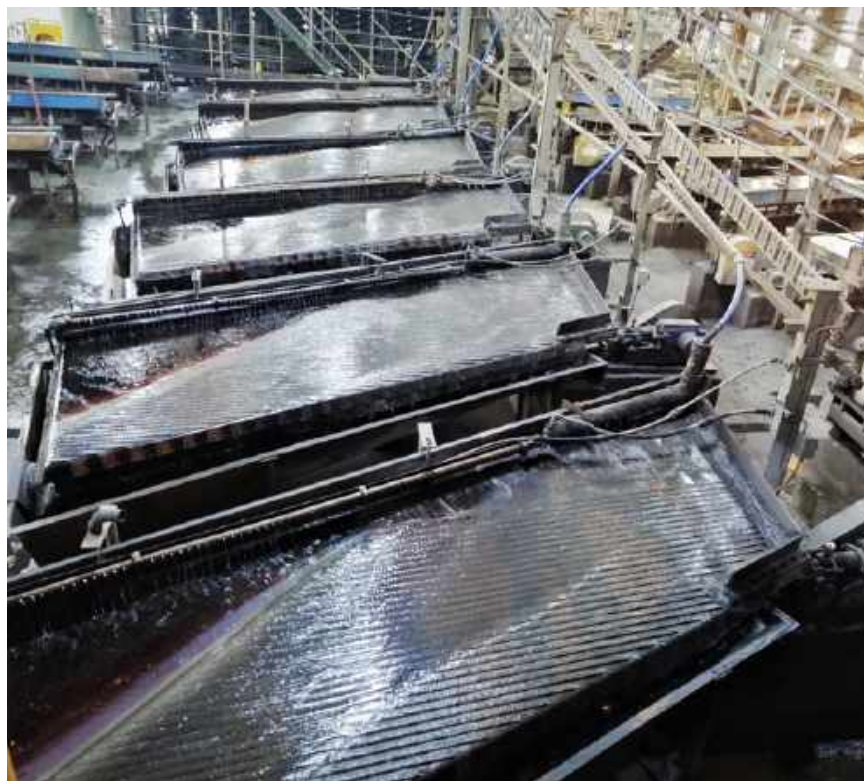
The Renison Processing Plant in western Tasmania uses gravity concentration for the recovery of tin; here some of the shaking tables used in this process are shown. The picture was taken during the November 2019 'Geometallurgy' Masters course.
