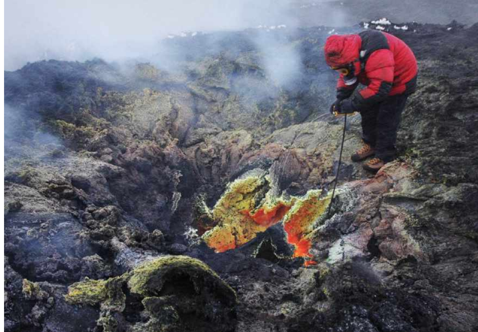
CODES collaborator and volcanologist Michael Zelenski performing measurements of temperature and composition of gas-air mixtures emitted through skylights and fractures in the roofs of lava tubes. This photograph accompanied an article in the journal Terra Nova (2019) by Professor Vadim Kamenetsky and colleagues entitled 'High-temperature gold-copper extraction with chloride flux in lava tubes of Tolbachik volcano (Kamchatka)'.
