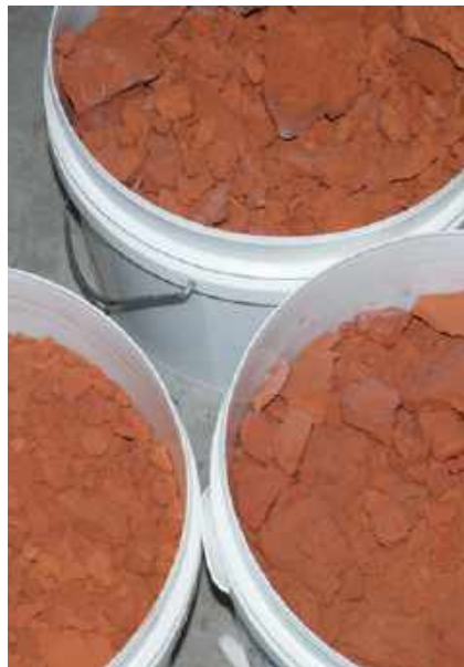
Buckets of red mud: bauxite refinery waste sourced from Bell Bay Aluminium in northern Tasmania is a potential acid mine/metalliferous drainage (AMD) ameliorant. PhD student Annah Moyo is researching its use in her project 'Utilising industrial waste materials for AMD control', which falls within TMVC Theme 3.
