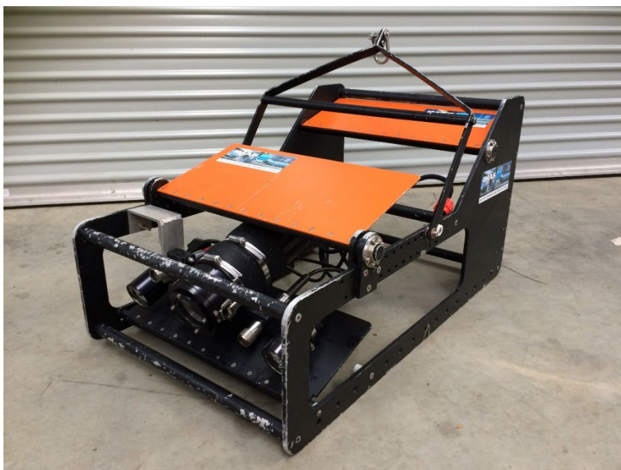
Figure 2. IMAS towed video camera unit.
