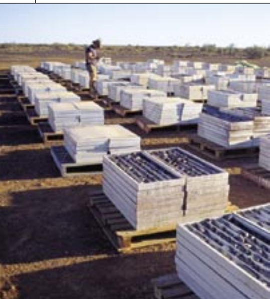
Bryan Bowden logging drill core at Prominent Hill, South Australia. (Project 4.8)
