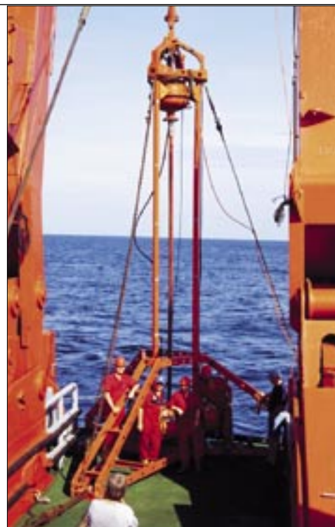
British Geological Survey 'Rockdrill' used to drill Conical Seamount and PACMANUS modern seafloor hydrothermal systems from the RV Sonne . (Project 3.8)
