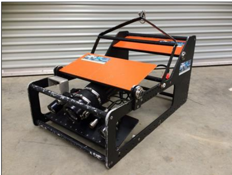
Figure 5. IMAS towed video camera unit.
